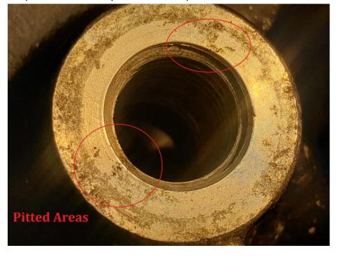
The bolt and banjo hose ends are more commonly a steel alloy, these will have small imperfections from manufacture which are concentric with the bores, essentially grooves and are less prone to pitting type corrosion. Aluminium alloy castings such as callipers and master cylinders are much more prone to pitting type surface imperfections over time.
