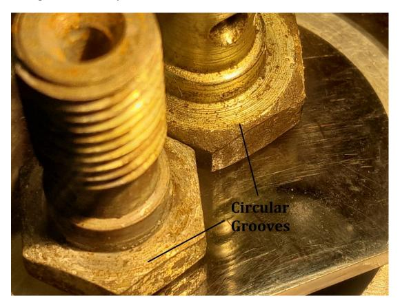
There is a technique that can help the sealing washer at the aluminium surface. First turn the forks against the steering stop away from the calliper you're working on, restrain the wheel or have an assistant hold them firmly. Next tighten the bolt to the recommended torque for that size. Take a drift / punch, prefferably of a softer material than the bolt, such as copper, brass or
