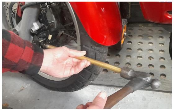
Now re-torque the bolt with the same setting, you will see that the bolt rotates slightly before it achieves the same torque as initial tightening. If you want to see how much difference this has made, mark along the length of the bolt / banjo to the calliper with a felt pen after the initial torque. In effect this will have applied enough additional longitudinal pressure to force the sealing washer/s to comply with the surface imperfections and hopefully a much better seal.
